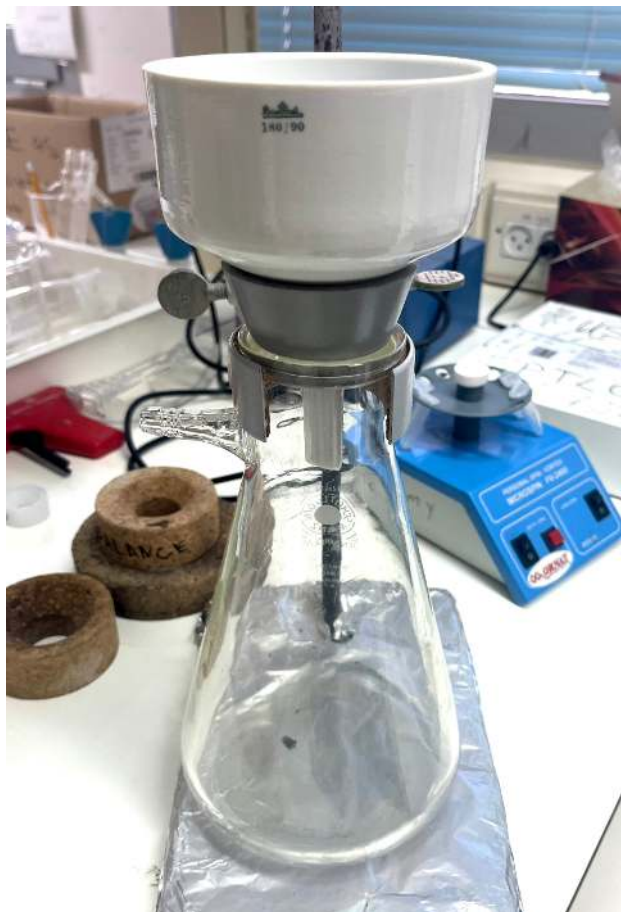
Filtration set-up with Buchner funnel
