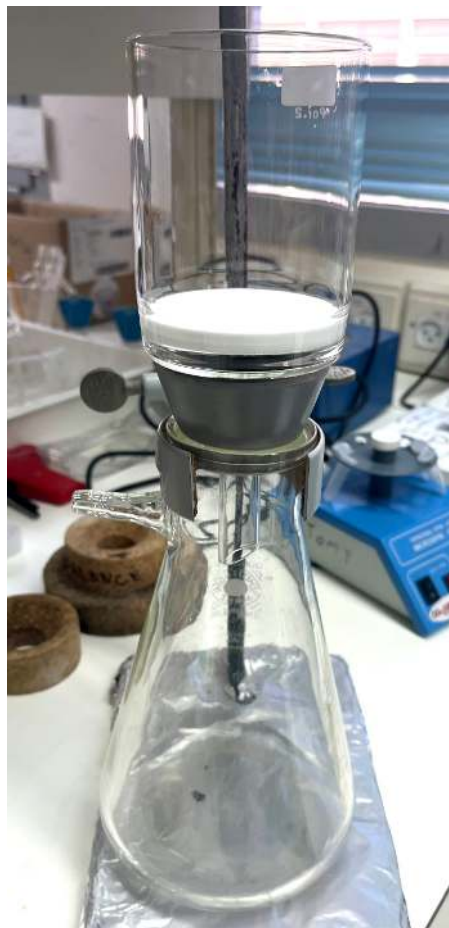
Filtration set-up with sintered funnel
